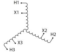
Three Phase Autotransformer with a capacity of 9kVA, transforming 550Y Volts to 230Y Volts
