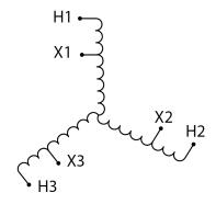
Three Phase Autotransformer with a capacity of 9kVA, transforming 480Y Volts to 220Y Volts
