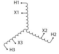
Three Phase Autotransformer with a capacity of 9kVA, transforming 480Y Volts to 220Y Volts
