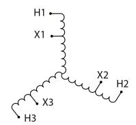
Three Phase Autotransformer with a capacity of 9kVA, transforming 120Y Volts to 440Y Volts
