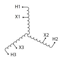
Three Phase Autotransformer with a capacity of 75kVA, transforming 220Y Volts to 575Y Volts
