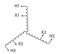
Three Phase Autotransformer with a capacity of 75kVA, transforming 220Y Volts to 240Y Volts
