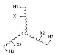
Three Phase Autotransformer with a capacity of 75kVA, transforming 208Y Volts to 575Y Volts
