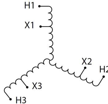
Three Phase Autotransformer with a capacity of 75kVA, transforming 200Y Volts to 416Y Volts
