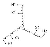
Three Phase Autotransformer with a capacity of 75kVA, transforming 120Y Volts to 440Y Volts
