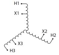
Three Phase Autotransformer with a capacity of 75kVA, transforming 120Y Volts to 115Y Volts
