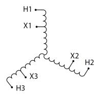
Three Phase Autotransformer with a capacity of 75kVA, transforming 115Y Volts to 380Y Volts
