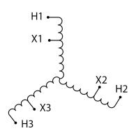
Three Phase Autotransformer with a capacity of 75kVA, transforming 115Y Volts to 347Y Volts
