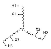
Three Phase Autotransformer with a capacity of 75kVA, transforming 115Y Volts to 220Y Volts
