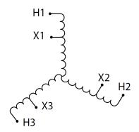
Three Phase Autotransformer with a capacity of 75kVA, transforming 110Y Volts to 575Y Volts
