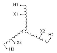
Three Phase Autotransformer with a capacity of 75kVA, transforming 110Y Volts to 480Y Volts
