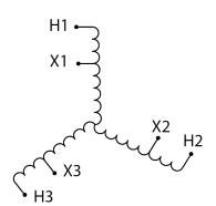
Three Phase Autotransformer with a capacity of 75kVA, transforming 110Y Volts to 416Y Volts
