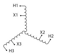
Three Phase Autotransformer with a capacity of 75kVA, transforming 110Y Volts to 415Y Volts
