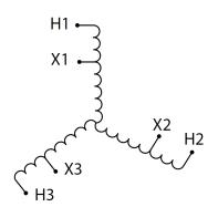
Three Phase Autotransformer with a capacity of 75kVA, transforming 110Y Volts to 277Y Volts
