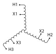
Three Phase Autotransformer with a capacity of 750kVA, transforming 120Y Volts to 575Y Volts
