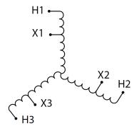
Three Phase Autotransformer with a capacity of 750kVA, transforming 115Y Volts to 575Y Volts
