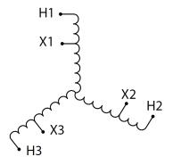
Three Phase Autotransformer with a capacity of 750kVA, transforming 115Y Volts to 460Y Volts
