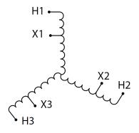
Three Phase Autotransformer with a capacity of 750kVA, transforming 110Y Volts to 416Y Volts
