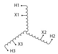
Three Phase Autotransformer with a capacity of 6kVA, transforming 600Y Volts to 440Y Volts
