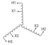
Three Phase Autotransformer with a capacity of 6kVA, transforming 440Y Volts to 480Y Volts
