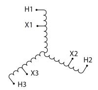
Three Phase Autotransformer with a capacity of 6kVA, transforming 220Y Volts to 110Y Volts
