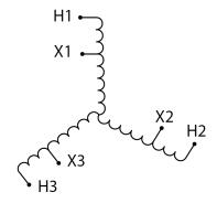
Three Phase Autotransformer with a capacity of 6kVA, transforming 120Y Volts to 400Y Volts
