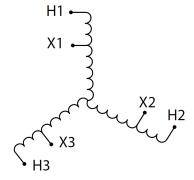
Three Phase Autotransformer with a capacity of 6kVA, transforming 115Y Volts to 277Y Volts
