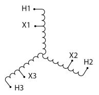
Three Phase Autotransformer with a capacity of 500kVA, transforming 416Y Volts to 200Y Volts
