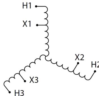
Three Phase Autotransformer with a capacity of 500kVA, transforming 200Y Volts to 550Y Volts
