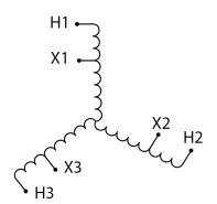
Three Phase Autotransformer with a capacity of 45kVA, transforming 600Y Volts to 208Y Volts
