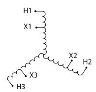
Three Phase Autotransformer with a capacity of 45kVA, transforming 575Y Volts to 277Y Volts
