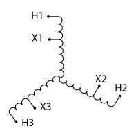
Three Phase Autotransformer with a capacity of 45kVA, transforming 480Y Volts to 115Y Volts
