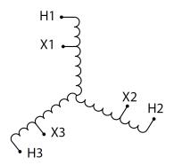
Three Phase Autotransformer with a capacity of 45kVA, transforming 460Y Volts to 277Y Volts
