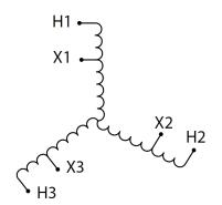
Three Phase Autotransformer with a capacity of 45kVA, transforming 440Y Volts to 550Y Volts
