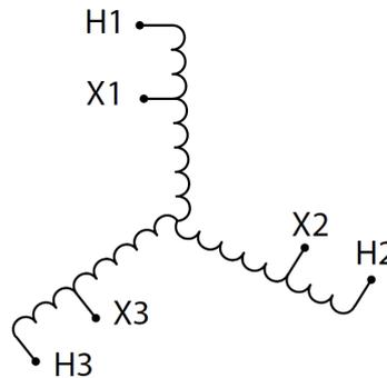
Three Phase Autotransformer with a capacity of 45kVA, transforming 415Y Volts to 480Y Volts
