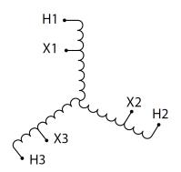
Three Phase Autotransformer with a capacity of 45kVA, transforming 415Y Volts to 380Y Volts
