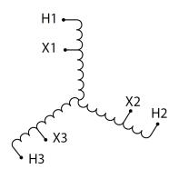
Three Phase Autotransformer with a capacity of 45kVA, transforming 415Y Volts to 208Y Volts
