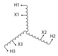
Three Phase Autotransformer with a capacity of 45kVA, transforming 277Y Volts to 120Y Volts
