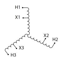
Three Phase Autotransformer with a capacity of 45kVA, transforming 240Y Volts to 575Y Volts
