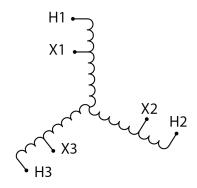
Three Phase Autotransformer with a capacity of 45kVA, transforming 240Y Volts to 110Y Volts
