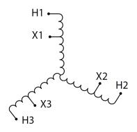
Three Phase Autotransformer with a capacity of 45kVA, transforming 230Y Volts to 480Y Volts
