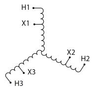
Three Phase Autotransformer with a capacity of 45kVA, transforming 220Y Volts to 380Y Volts
