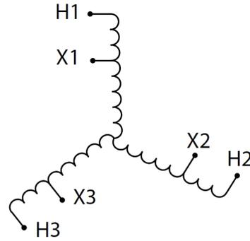
Three Phase Autotransformer with a capacity of 45kVA, transforming 220Y Volts to 208Y Volts
