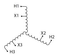
Three Phase Autotransformer with a capacity of 45kVA, transforming 208Y Volts to 480Y Volts
