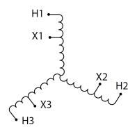
Three Phase Autotransformer with a capacity of 45kVA, transforming 208Y Volts to 415Y Volts
