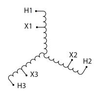
Three Phase Autotransformer with a capacity of 45kVA, transforming 208Y Volts to 230Y Volts
