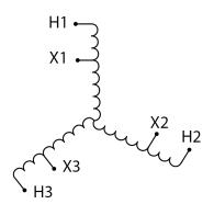
Three Phase Autotransformer with a capacity of 45kVA, transforming 200Y Volts to 440Y Volts
