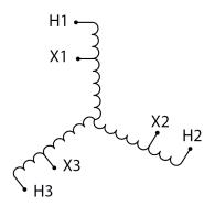
Three Phase Autotransformer with a capacity of 45kVA, transforming 200Y Volts to 120Y Volts
