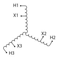
Three Phase Autotransformer with a capacity of 45kVA, transforming 120Y Volts to 380Y Volts
