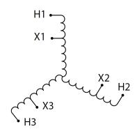
Three Phase Autotransformer with a capacity of 45kVA, transforming 120Y Volts to 347Y Volts
